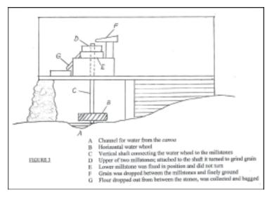
Raw grain was dropped from a chute at F into the area between the millstones, where it was finely ground. The resulting flour was then collected at point G, and bagged for use.
